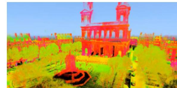
The georeferenced dataset: photos and LiDAR data acquired by Stereopolis, the IGN mobile scanning vehicle
